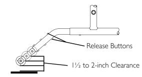
FIGURE 9.3 Adjusting the Anti-Tippers
